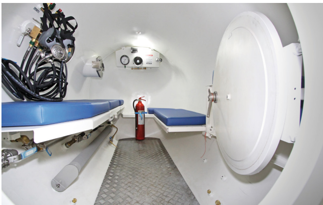
Deck Decompression Chamber
